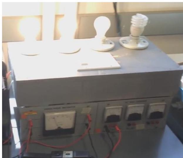
Figure 2.2: Switching load power to observe current supply behavior
