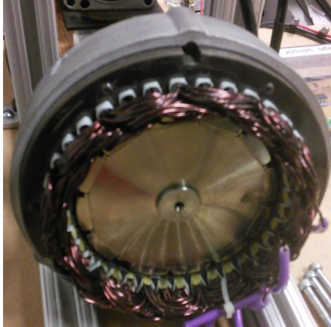
Figure 1.8: Permanent magnet synchronous generator from 2008 Air-X 400W wind Turbine
