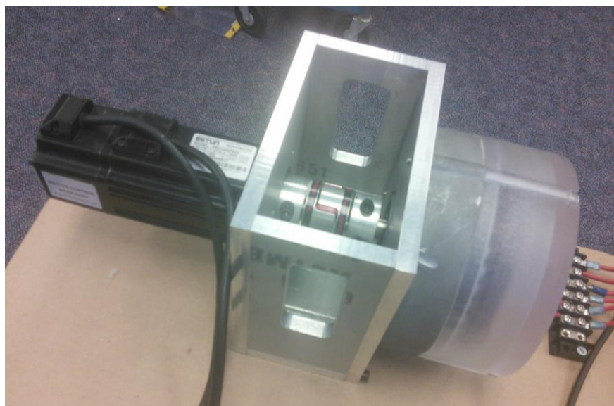
Figure 1.11: New CNC machined custom coupling mount assembled
